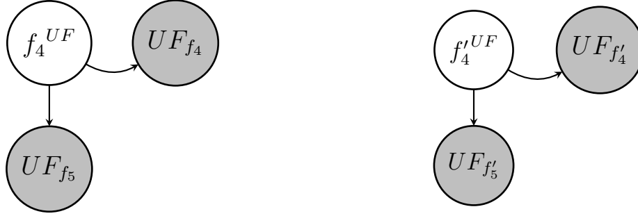
Figure 4.9: Call graphs of the isolated versions of f_4 and f'_4 when \langle f_2, f'_2 \rangle \notin S . The same UF, UF', which respectively replace calls to f_5, f'_5 and f_4, f'_4 , are distinguished as UF_{f_5}, UF_{f'_5} and UF_{f_4}, UF_{f'_4} , respectively, for better understanding.
