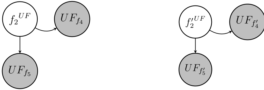
Figure 4.6: Call graphs of the isolated versions of f_2 and f'_2 . Partially equivalent UF, UF', which respectively replace calls to f_5 , f'_5 and f_4 , f'_4 , are distinguished as UF_{f_5}, UF_{f'_5} and UF_{f_4}, UF_{f'_4} , respectively, for better understanding.
