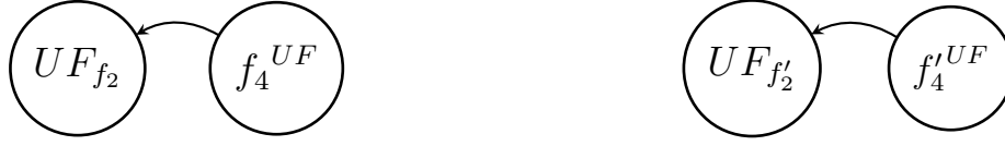
Figure 4.7: Call graphs of the isolated versions of f_4 and f'_4 . UF and UF' , which replace calls to f_2 and f'_2 , respectively, are distinguished with UF_{f_2} and UF_{f'_2} , respectively, for better understanding. They emulate different uninterpreted functions.
