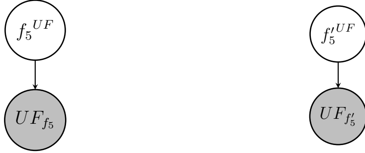
Figure 4.4: Call graphs of the isolated versions of f_5 and f'_5 . UF_{f_5} and UF_{f'_5} , which have replaced the calls to f_5 and f'_5 , respectively, emulate the same uninterpreted functions and are marked gray.
