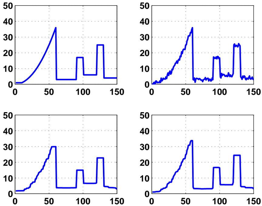
Figure 2: Top left: original signal. Top right: noisy signal ( $\sigma = 0.9$ , PSNR=25.32 db). Bottom left : ROF reconstruction. (PSNR=27.09 db). Bottom right: Signal reconstructed using windows ( $\mu_1 = 1000$ ,  $\mu_2 = 0.02$ , PSNR=28.89 db).
